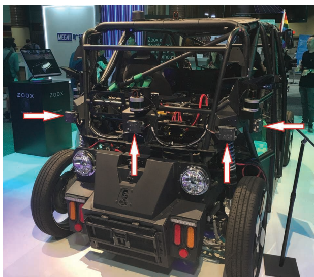
FIGURE 1. A Zoox autonomous driving vehicle, exhibited at the 2019 Conference on Computer Vision and Pattern Recognition, is equipped with 10 millimeter-wave (mm-wave) automotive radar sensors (marked by white arrows) at the front, rear, left, and right sides.
